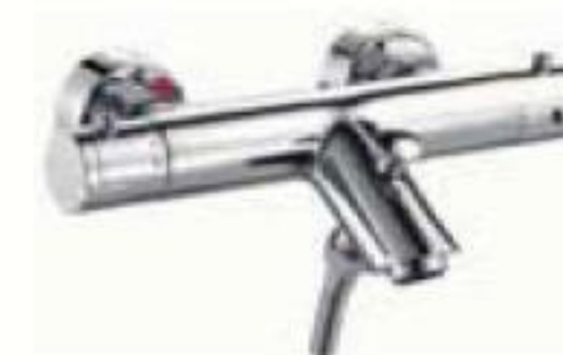
1001ST3 Thermostatic bath/shower mixer 1/2" outlet hose connection 38°C±1°C safe temperature stop Wall cap and s-connector
